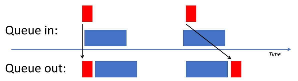
The Maximum QOS priority inversion delay is the *output port wire speed time of a full size packet* multiplied by the *number of switches* the high priority packet passes through.
