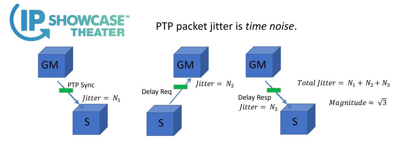
An audio clock recovered from PTP using peer delay will be less stable than an audio clock recovered from only the PTP sync packets.
